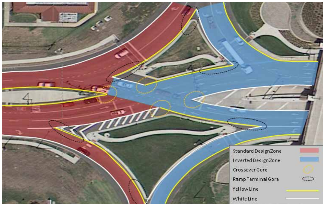
Exhibit 8-20. Example centerline and edge line pavement markings at a DDI. Ramp terminal gore areas will transition from 12-inch white gore markings to standard edge lines. (26)
