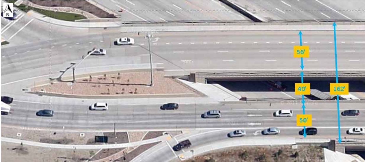
Exhibit 7-13. Cross-sectional distances for a shifted alignment with no reverse curves between crossovers (Pioneer Crossing, American Fork, UT). (26)
