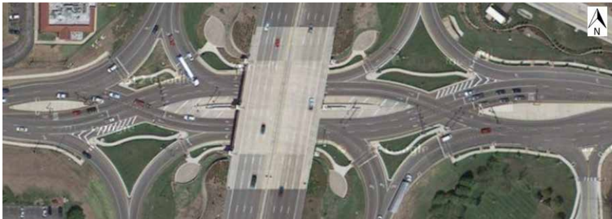
Exhibit 7-10. Symmetrical alignment with no reverse curves between crossovers (Dorsett Road, Maryland Heights, MO). (26)
