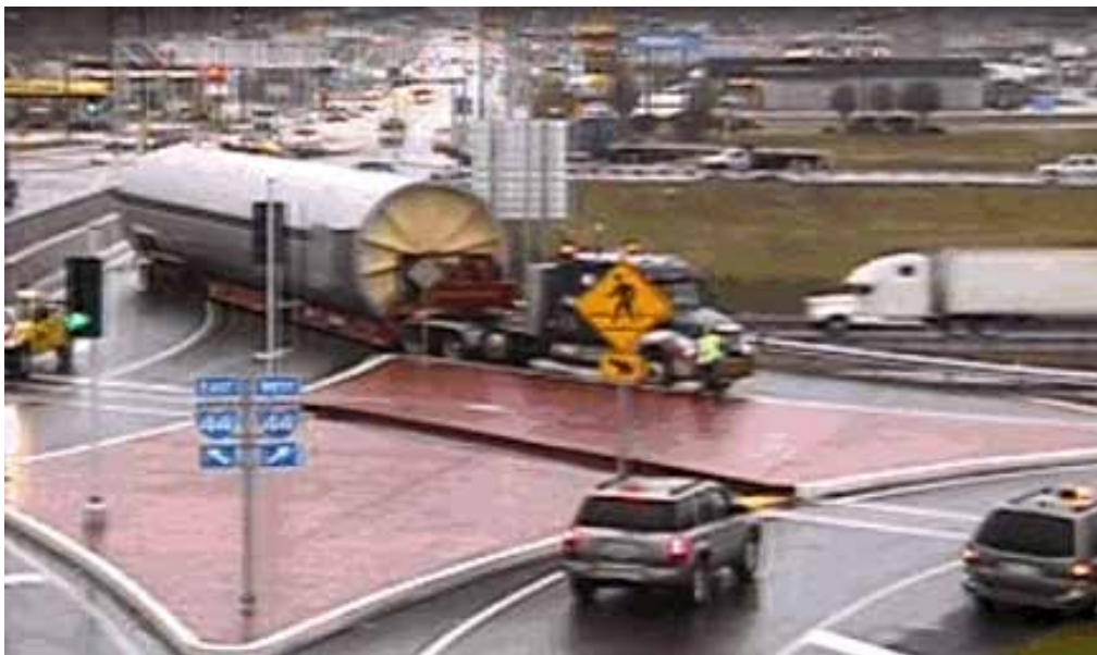
Exhibit 7-5. An oversized load making a left turn onto I-44 at MO 13 (Springfield, MO). (16)
