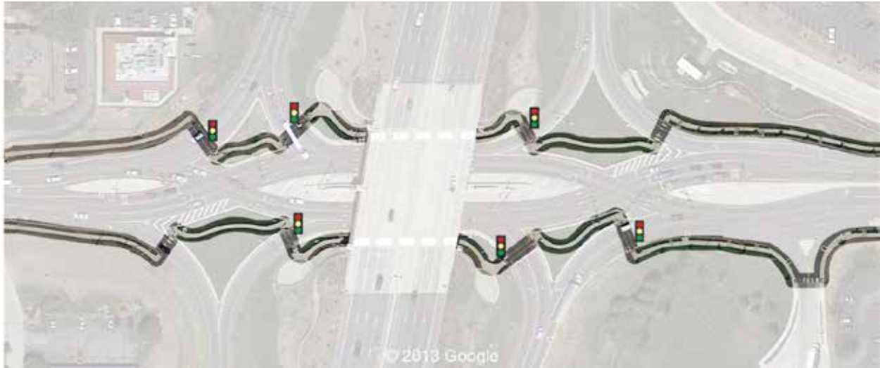
Exhibit 3-6. Pedestrian facilities on outside of DDI (Maryland Heights, MO). (26)
