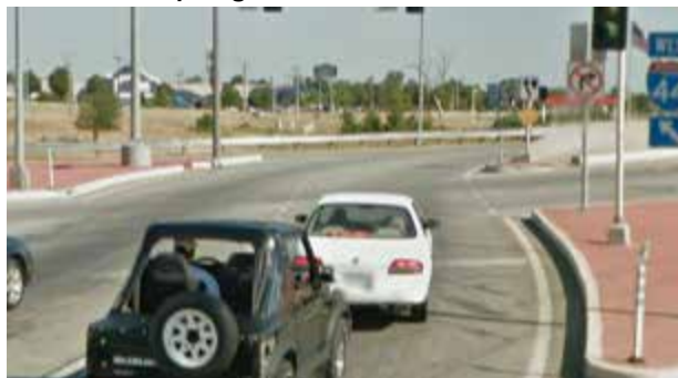
Exhibit 7-15. Barriers and traffic islands to discourage wrong-way movements. (26)
