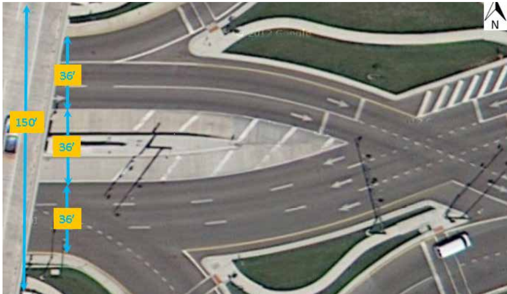
Exhibit 7-11. Cross-sectional distances for a symmetrical alignment with no reverse curves between crossovers (Dorsett Road, Maryland Heights, MO) (26)
