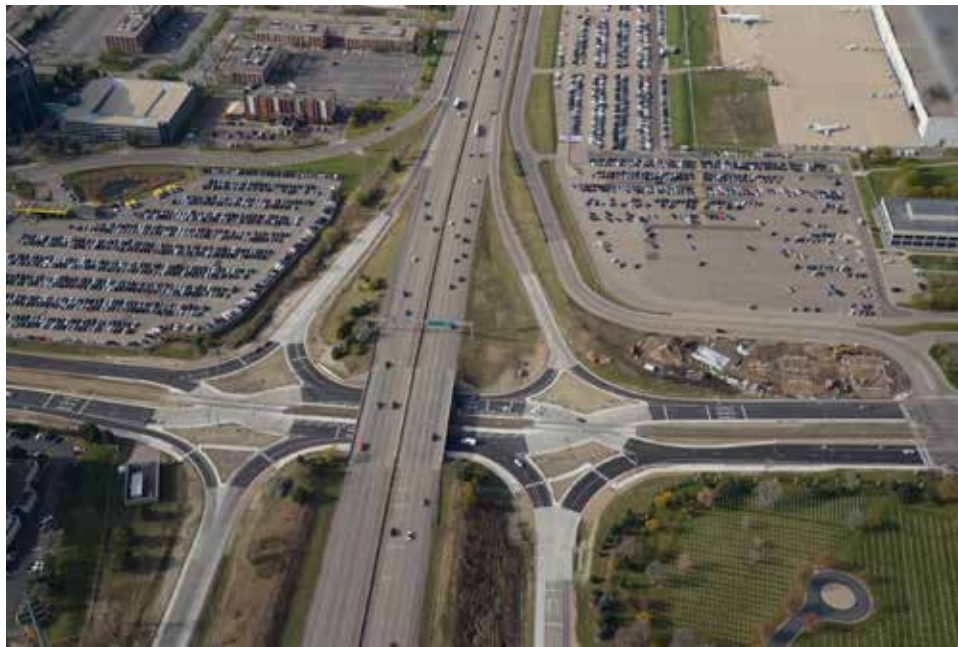
Exhibit 3-28. Aerial view of DDI with center-running light rail at I-494 and 34th Avenue in Bloomington, MN. (29)
